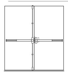
Mortise lock and surface mounted or Concealed Vertical rod device combination—same direction
