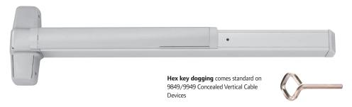
**9849/9949 concealed vertical cable device** for use on single or metal doors, UL listed for Panic Exit Hardware. Devices are ANSI A156.3 – 2001 Grade 1. The 9849 device has a smooth mechanism case and the 9949 device has a grooved case. The concealed vertical cable device is non-handed except when the following device options are used: SD (Special Dogging), or SS (Signal Switch). See Opposite page for available outside trim and device functions.
