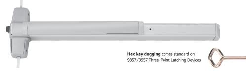
**9857/9957 three-point latching device** for all types of single or double doors, UL listed for Panic Exit Hardware. Devices are ANSI A156.3 – 2001 Grade 1. Covers stock hollow metal doors with 86 or 161 cutouts. The 9857 device has a smooth mechanism case and the 9957 device has a grooved case. The three-point latching device is non-handed except when the following device options are used: SD (Special Dogging), or SS (Signal Switch). See Opposite page for available outside trim and functions.
