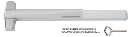
9848/9948 Concealed vertical rod device for use on single or double metal doors, UL listed for Panic Exit Hardware. Covers stock hollow metal doors with 86 or 161 cutouts. Devices are ANSI A156.3 – 2001 Grade 1. The 9848 device has a smooth mechanism case and the 9948 device has a grooved case. The concealed vertical rod device is non-handed except when the following device options are used: SD (Special Dogging), or SS (Signal Switch). See Opposite page for available outside trim and functions.
