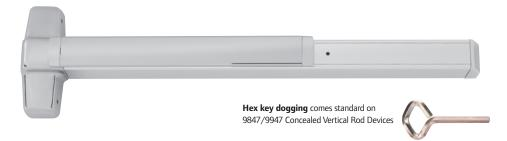
**9847/9947 concealed vertical rod device** for use on single or double metal doors, UL listed for Panic Exit Hardware. Devices are ANSI A156.3 – 2001 Grade 1. The 9847 device has a smooth mechanism case and the 9947 device has a grooved case. The concealed vertical rod device is non-handed except when the following device options are used: SD (Special Dogging), or SS (Signal Switch). See Opposite page for available outside trim and device functions.
