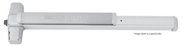
Braille touchpad embossed with the standard message "CAUTION STAIRWELL" in braille and raised letters provides assistance to persons with impaired vision. Letters are  $\frac{1}{2}$ " (13mm) high and braille is #2, raised height is  $\frac{3}{2}$ " (2mm). Other messages are available on special order, limited to 20 characters per line.\* - To order, specify: Suffix BR, EL9927L-BR
